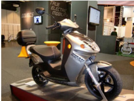
The scooters are using high efficiency and sophisticated brushless motors with a low-wear belt drive which makes the machines much lighter.
